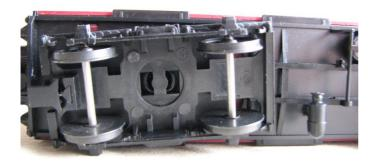
Re wheeled bogie. EM wheels used in Picture
